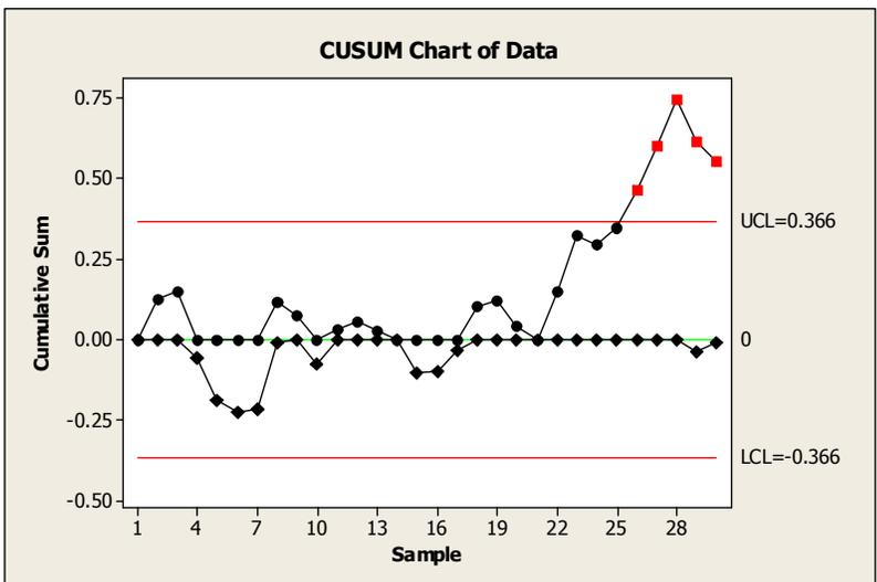
Note that the CUSUM chart actually plots cumulative sums in each direction (positive and negative) independently. In this case, the process change is detected on the 6<sup>th</sup> sample following the process “shift.” While the computation of the individual CUSUMs
