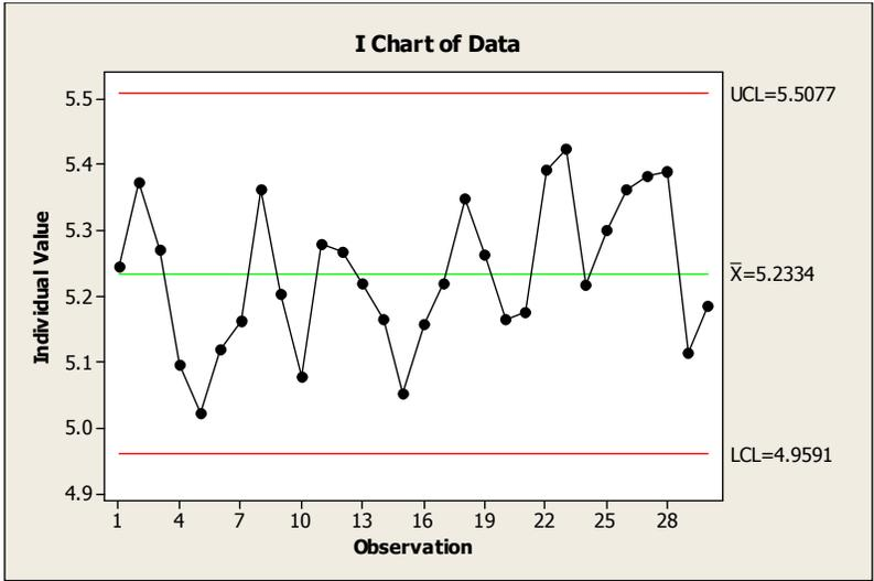
It is not apparent that any process shift has occurred after sample 20. No points exceed a control limit and no run or trend rules are violated. Even if a run rule was violated (and the user is applying run rules to the chart), a run of 7 (or 8 or 9) consecutive points above the centerline would be required which would mean that the earliest that the shift could be detected is on sample 27.
