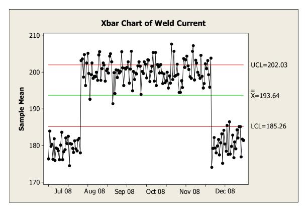
During the problematic production periods (Aug 08 - Nov 08), the weld current was running around 195 Amps on average vs. around 180 Amps during months when few failures occurred. This picture along with the results of the designed experiment confirmed that high weld currents caused low weld strengths which then led to the costly field failures.
