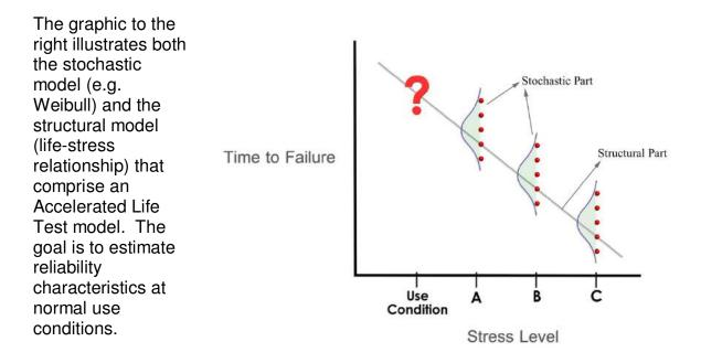
The structural model which describes the life-stress relationship may be determined empirically from the data, but knowledge of the *physics of failure* and underlying failure mechanisms is desired. This knowledge helps to justify the use of a specific model form and extrapolation to normal use conditions (as extrapolation always introduces risk into predictions).
